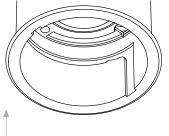
Reflector can be rotated 90° to ensure proper alignment. Friction-fit design maintains installation integrity.
